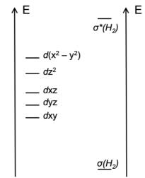
Figure 1: Simplified diagram of molecular orbitals of the Kubas complex
