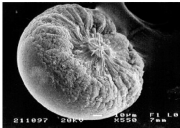
Fig. 4. SEM image showing half of an equatorially notched fluoroapatite-gelatin spheroid. Scale bar is 10 µm. Reproduced with permission from Chemistry of Materials [30]. Copyright 2001 American Chemical Society.
